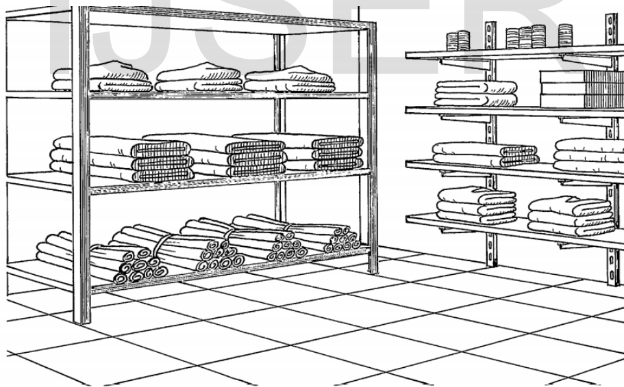
Figure 7: Multi-level racks save space and allow material to be temporarily stored in an orderly manner
